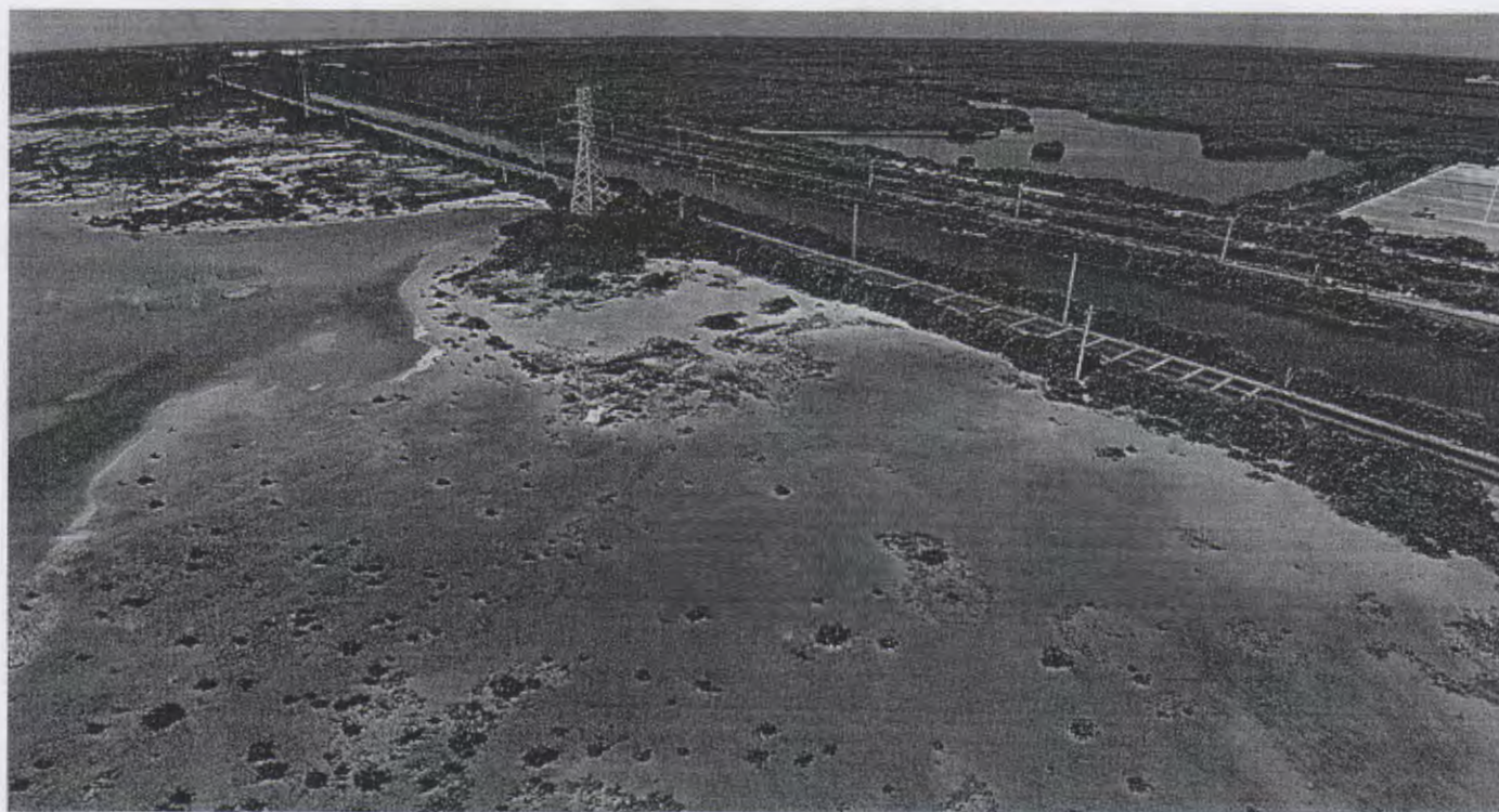
Fig. 28.1 Road that crosses the mangrove and the impact caused by the interruption of water flows
